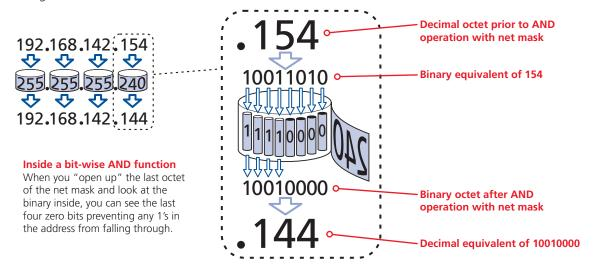
Thus, when 154 is *bit-wise ANDed* with 240, the result is 144. Likewise, any local address from 192.168.142.**144** through to 192.168.142.**159** would produce exactly the same result when combined with this net mask, hence they would all be local addresses. However, any difference in the upper three octets or the upper four bits of the last octet would slip through the mask and the address would be flagged as not being local.
